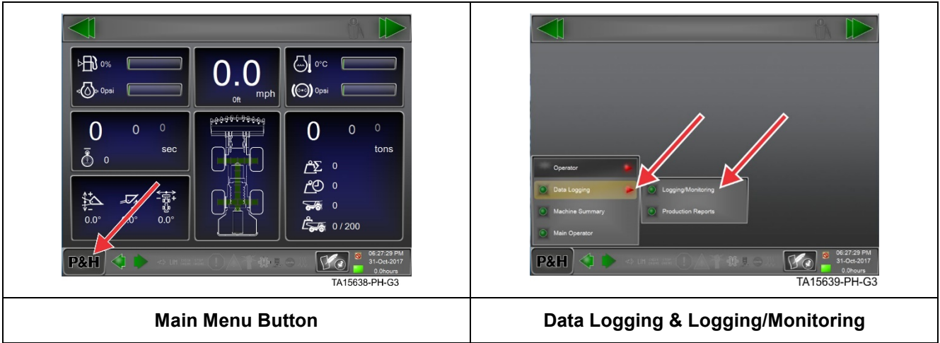
LINCS logging/monitoring menu access
