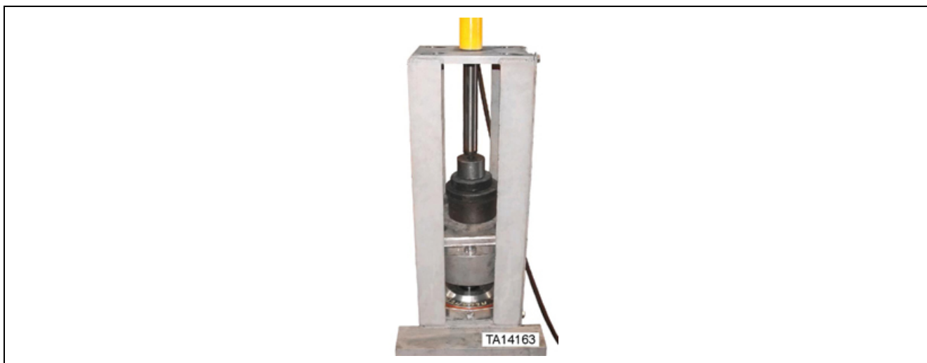
Figure 59. Pressing inner canister for final assembly (1 of 2)
