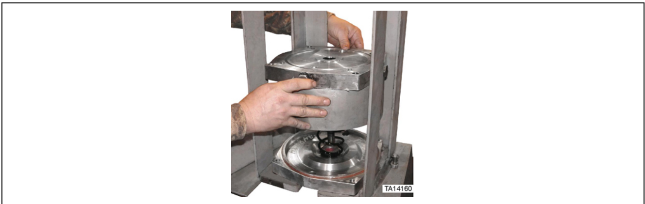
Figure 56. Positioning of top side inner end cap for pressing
