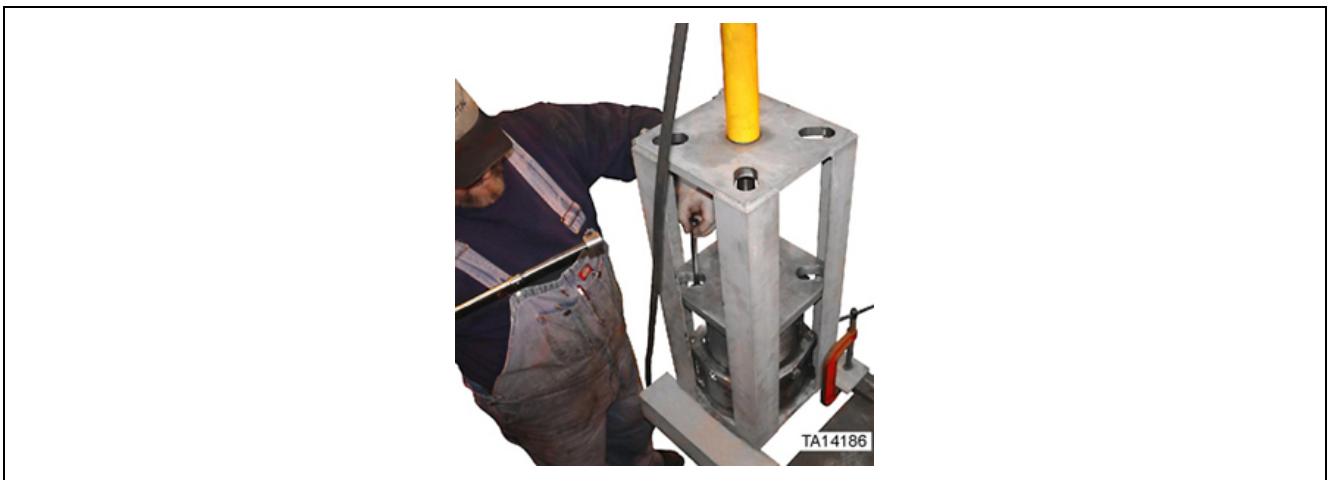
Figure 38. Removal of bolts securing end cap (2 of 2)
