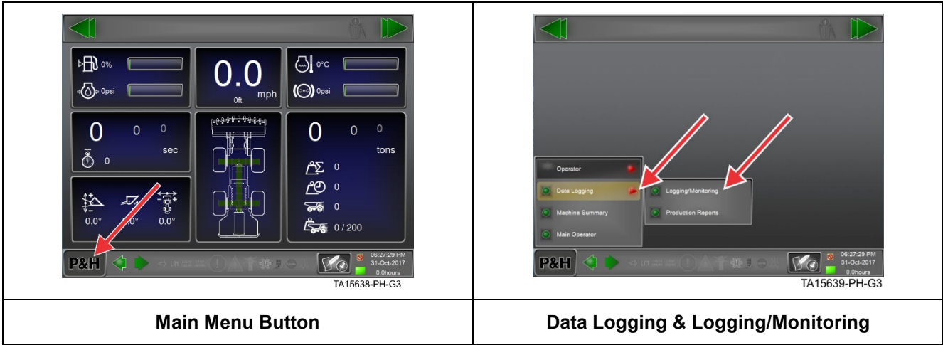
Figure 12. LINCS logging/monitoring menu access
