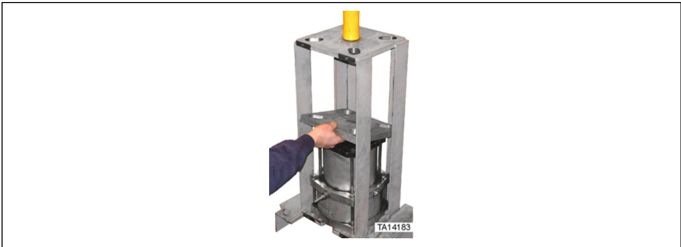
Figure 35. Placing press plate into press
