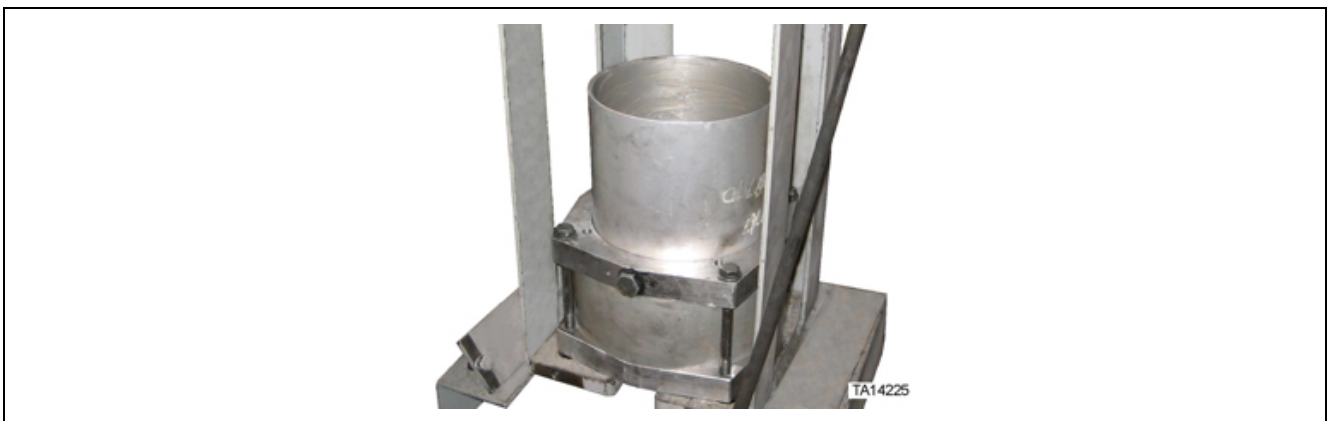
Figure 67. Outer housing in position in press
