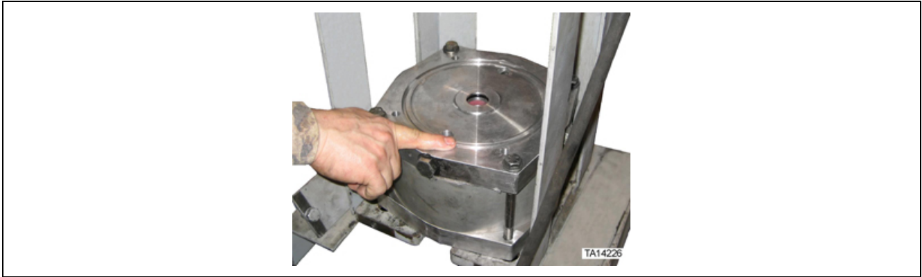
Figure 65. Lubrication of inner end cap for installation of O-ring
