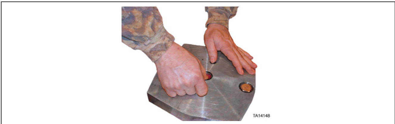
Figure 45. Installation of O-ring to end cap
