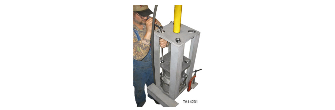
Figure 70. Installation of bolts securing outer housing
