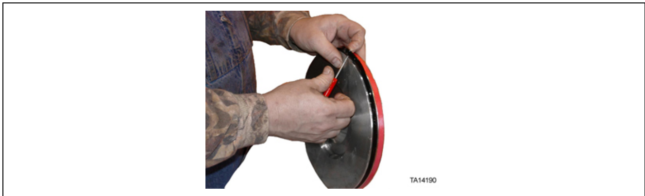
Figure 42. Removal of seals and wear rings (1 of 2)
