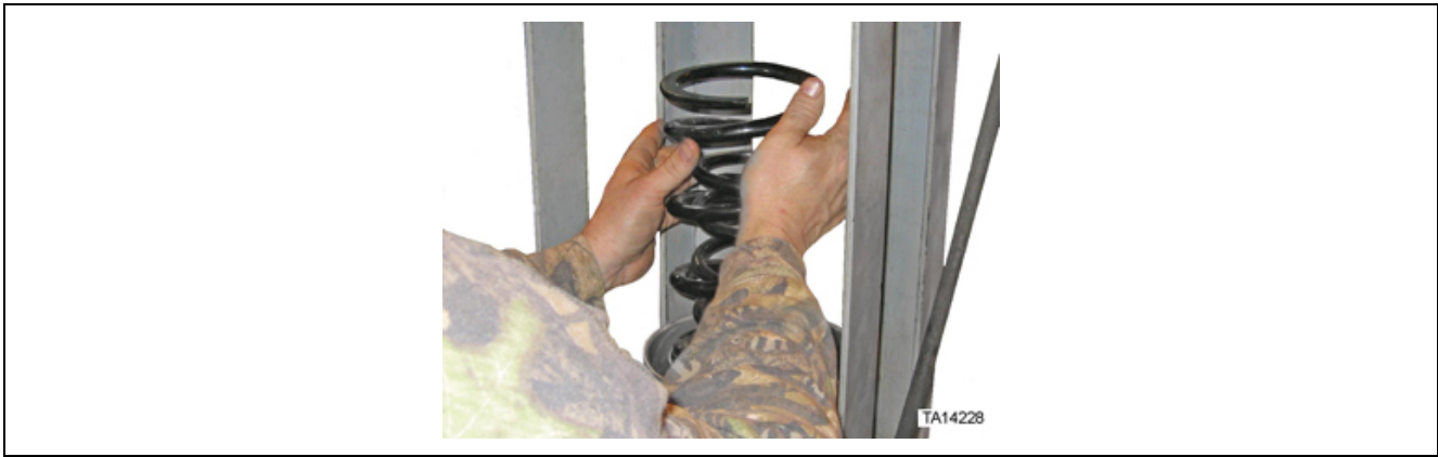
Figure 68. Installation of spring assembly into housing
