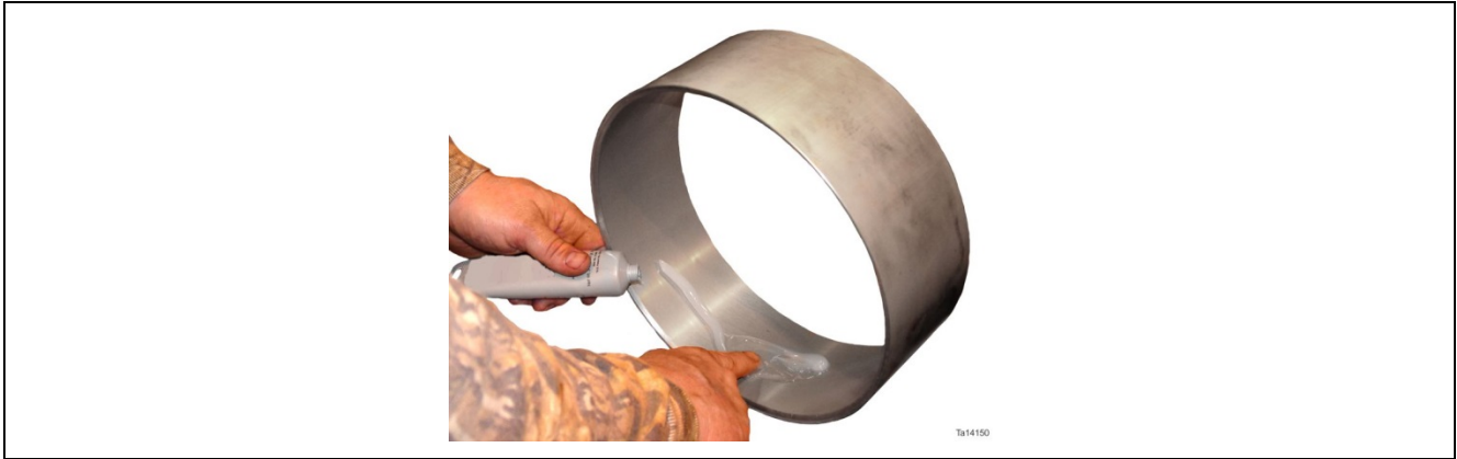
Figure 49. Lubrication of inner housing
