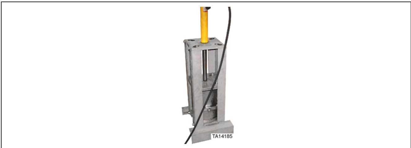
Figure 36. Press ram seated against press plate
