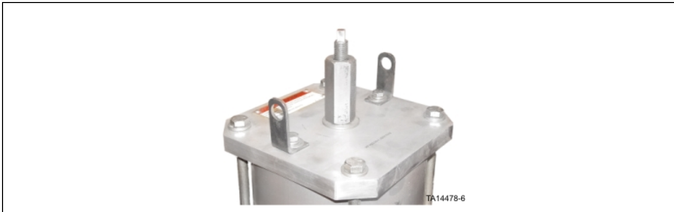
Figure 26. View of jack rod installed in brake cylinder
