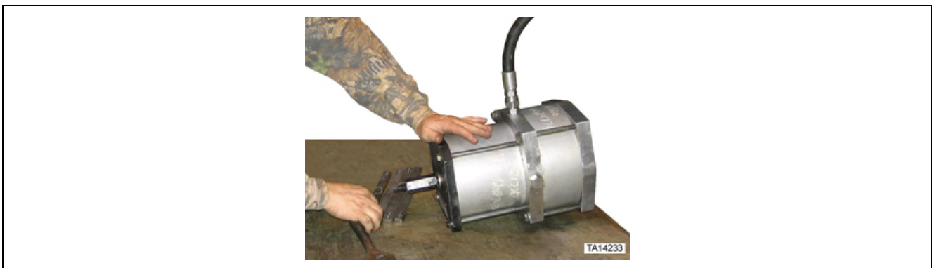
Figure 72. Use of jack bolt to release park brake to test actuator operation
