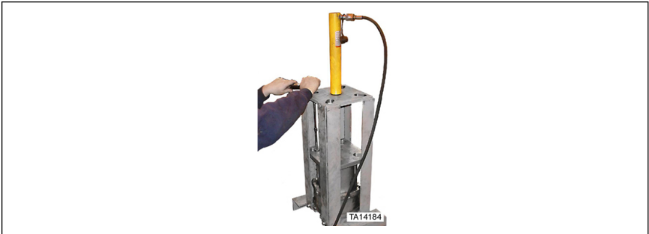
Figure 37. Removal of bolts securing end cap (1 of 2)
