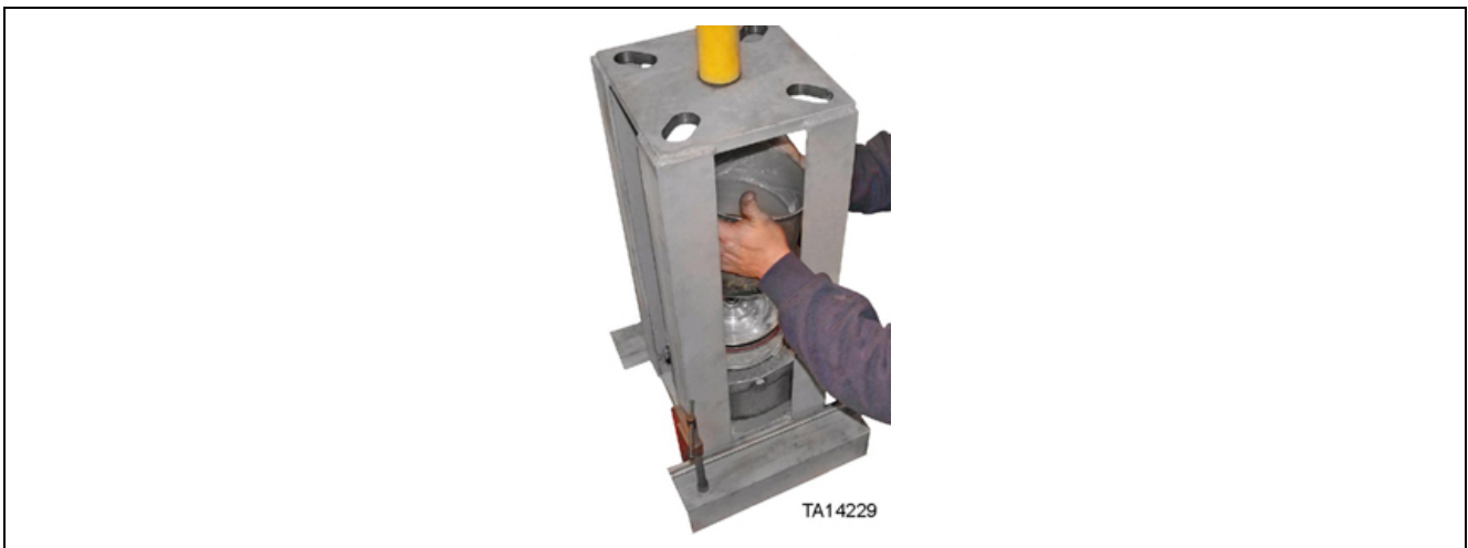
Figure 66. Installation of outer housing
