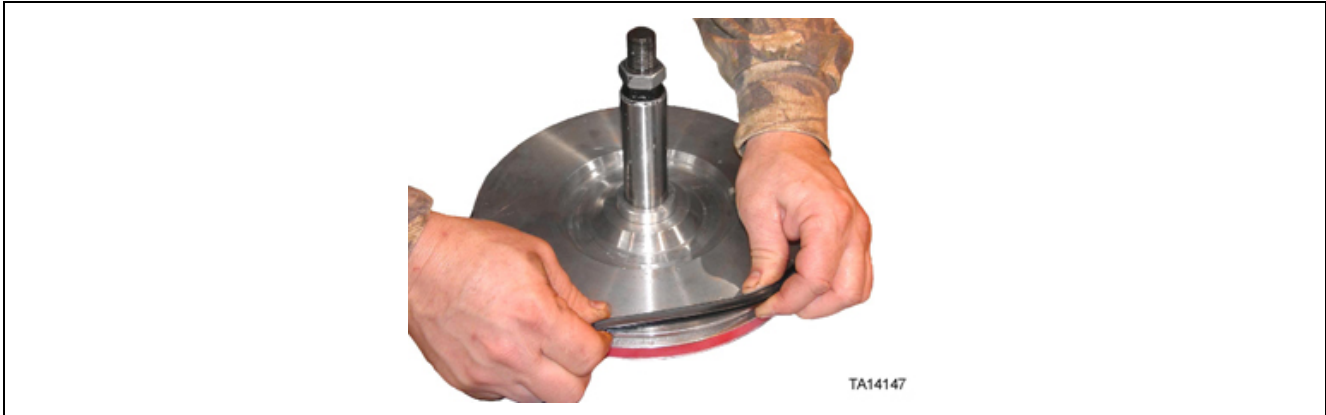
Figure 44. Installation of seal and wear ring to piston
