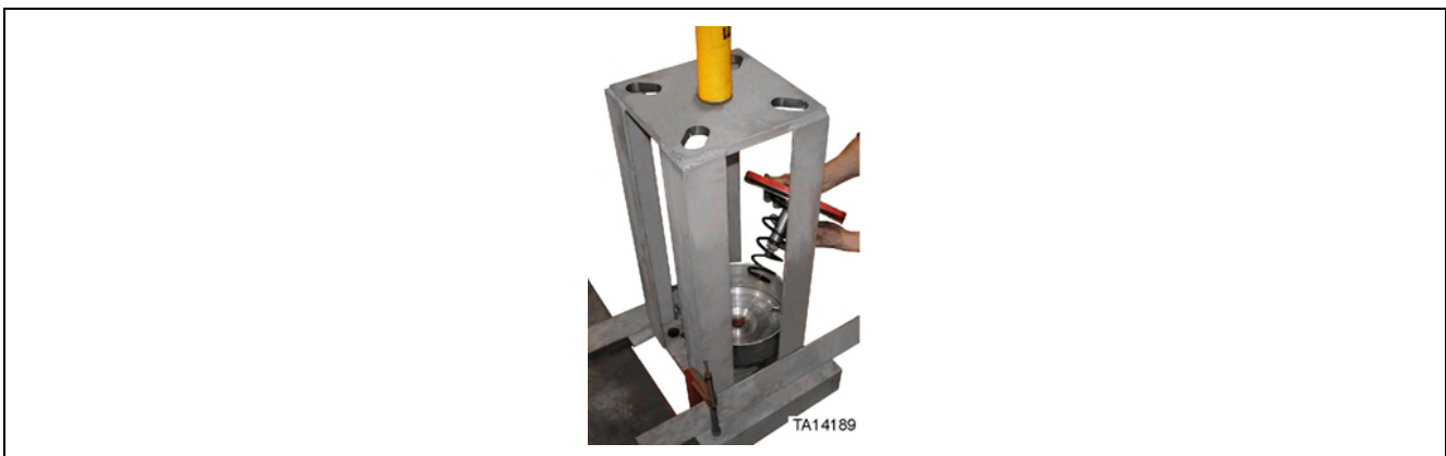
Figure 41. Removal of inner spring and piston
