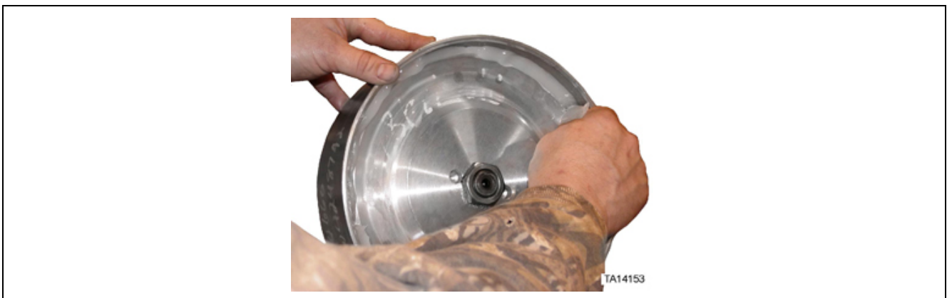
Figure 51. Lubrication of piston in inner housing
