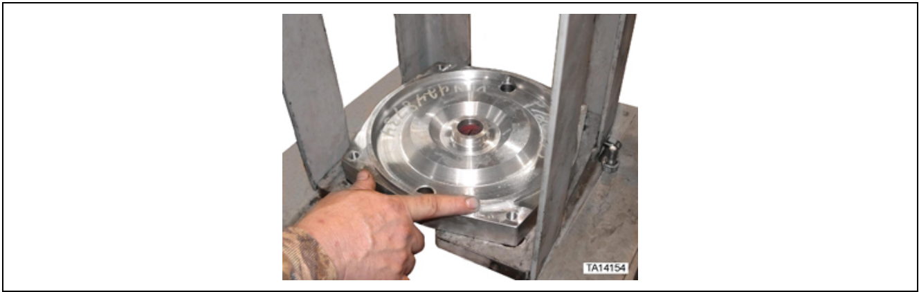
Figure 46. Lubrication of inner end cap for installation of O-ring
