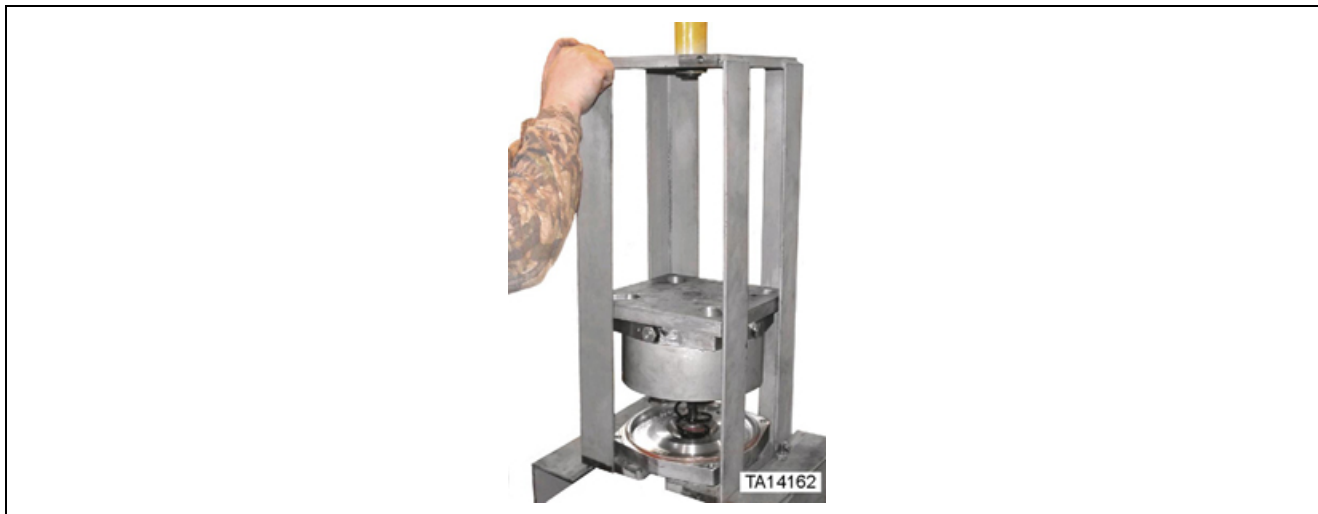
Figure 58. Installation of safety plates prior to final assembly of inner canister
