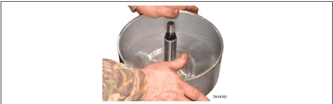
Figure 50. Installation of piston into inner housing
