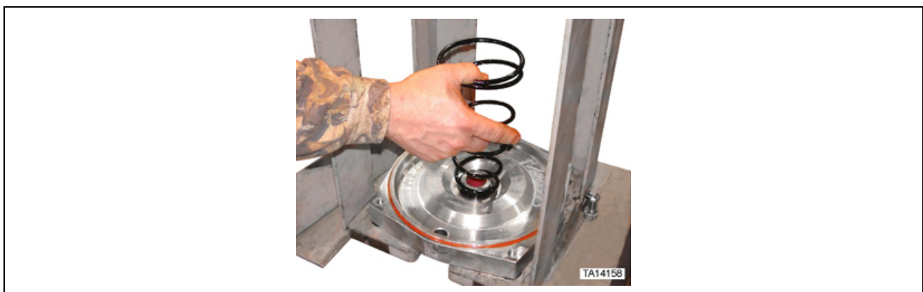
Figure 54. Installation of spring onto inner end cap
