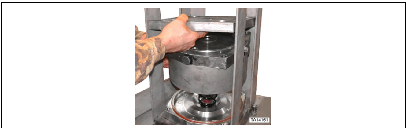
Figure 57. Placement of press plate into press for final assembly of inner actuator
