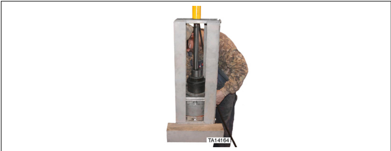
Figure 60. Pressing inner canister for final assembly (2 of 2)
