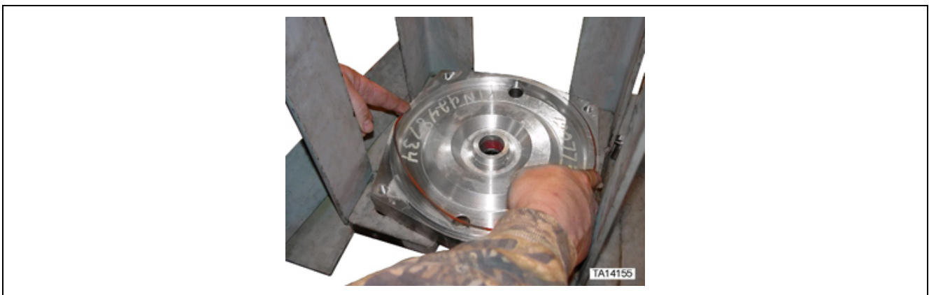
Figure 47. Installation of O-ring on inner end cap
