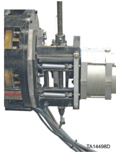
Figure 32. Positioning of pipe clamp for adjustment of torque tube
