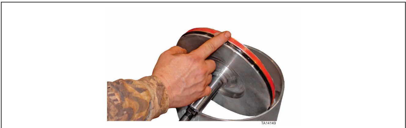
Figure 48. Lubrication of seal and wear ring
