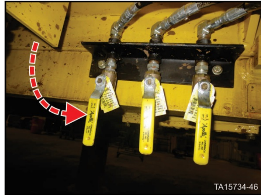
Figure 10. Open air reservoir bleed valves
