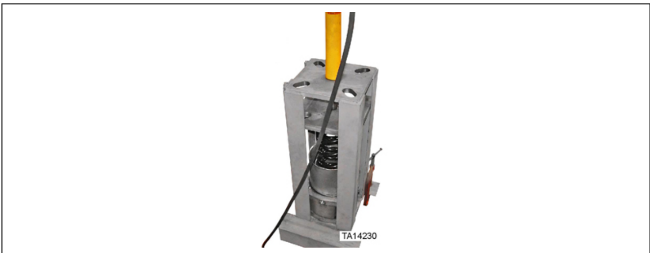
Figure 69. Compression of outer housing components
