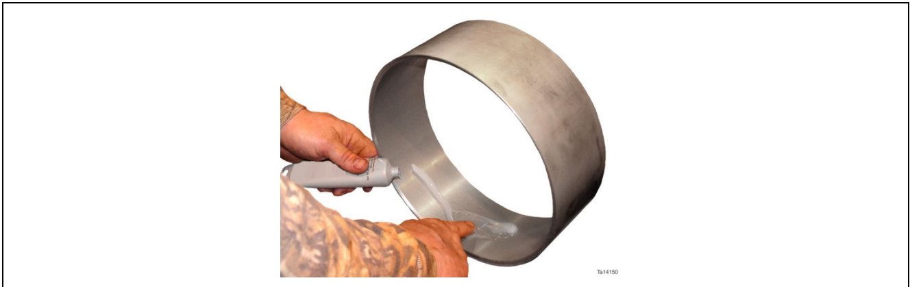
Figure 63. Lubrication of inner housing
