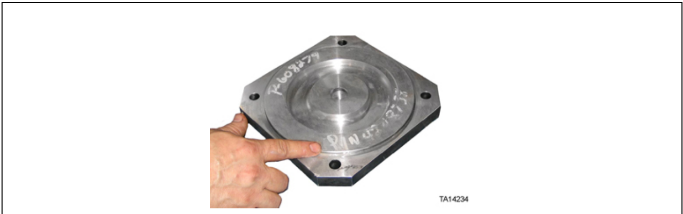
Figure 64. Lubrication of end cap installation of O-ring
